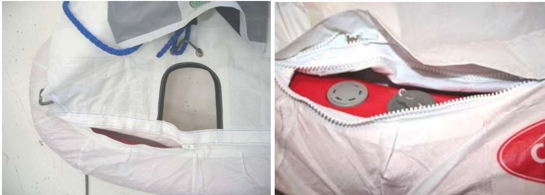
Unzip the chafe-guard to expose the valves
